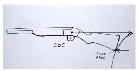
In the first phase of recoil, the gun travels to the rear and then encounters the firm resistance of the shooters shoulder, then, during the second phase of recoil, the gun rotates upward using the shooters shoulder as a pivot as shown in this picture.
