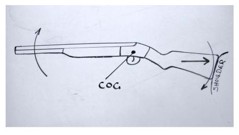
The way a shotgun recoils can be divided into two periods. The center of gravity of a shotgun is not along the axis of the bores but underneath the axis of the bores as shown in this diagram on the left. If the center of gravity was along the axis of the bores, the gun would recoil in a rearward direction only.
